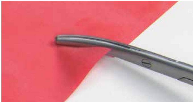
PHOTO A: Scissors cut cleanly through to the tip. No snagging or catching indicates that the scissor is surgically sharp.
